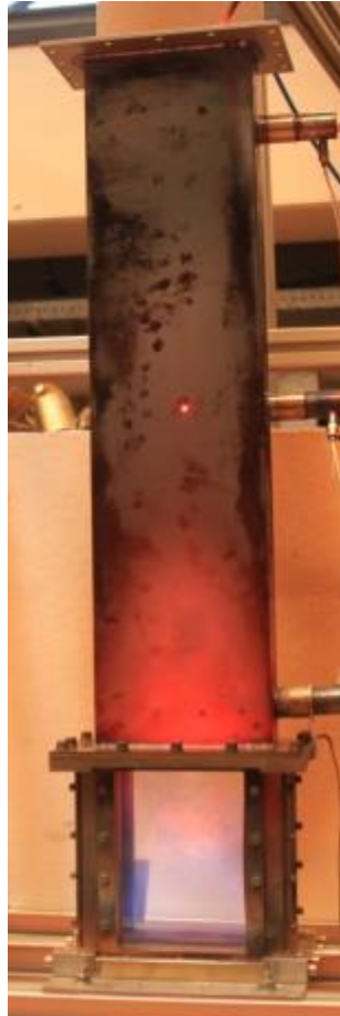
Figure 5-1: The LIMOUSINE combustor: thermal load on the structure in an unstable operating condition. Red dot on structure center is the laser vibrometer beam
